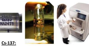
Self-shielded irradiators (research and blood processing), and calibrators (dosimeter and detector calibration)
